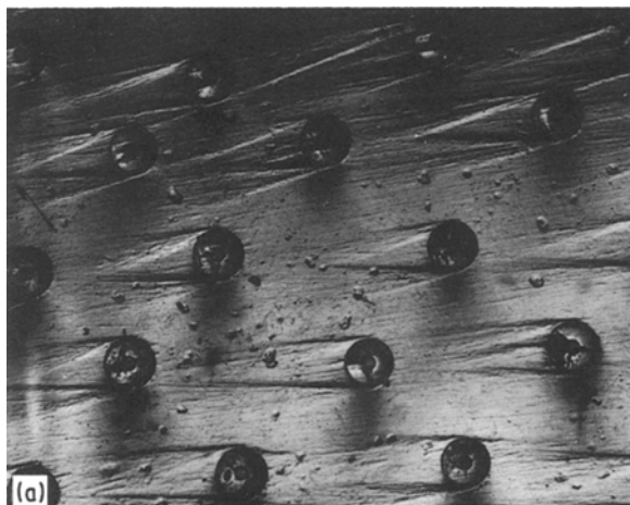
Figure 2 A composite specimen with perfectly aligned fibres after matrix infiltration, (a) cross-sectional view, and (b) top view.
